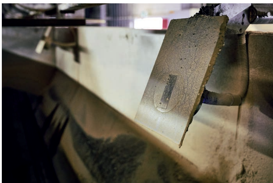
Solitrend ensures fast and reliable measurement of moisture directly in bulk solid flows.
